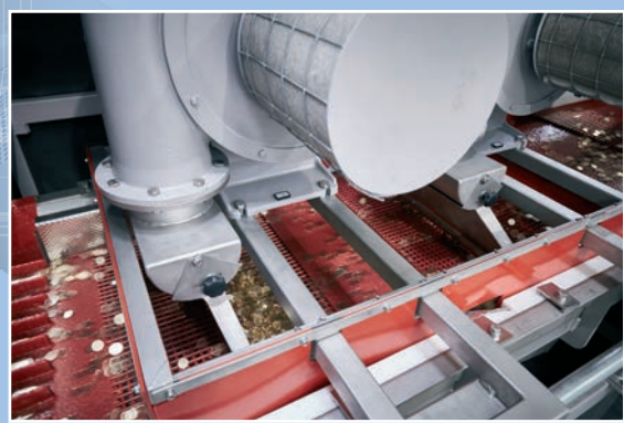
Water removal prior to drying
